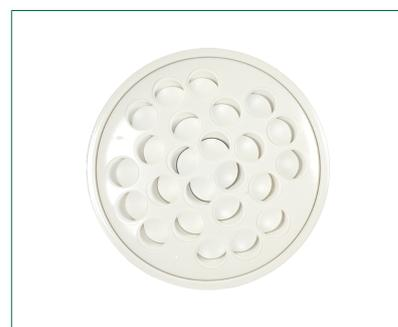
The DYRB is a quiet, ceiling-mounted supply air unit that consists of a nozzle diffuser, DYRH, and a plenum box, ATTD. The diffuser has adjustable nozzles for the setting of an optional diffusion pattern. The slot height of the diffuser can be set at 0 or 12 mm. Fixed to the diffuser body with magnets, the diffuser plate is easy to open. The DYRH nozzle diffuser is also available without the plenum box.
